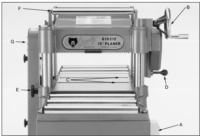
Figure 9. Overview of planer adjustment controls.
